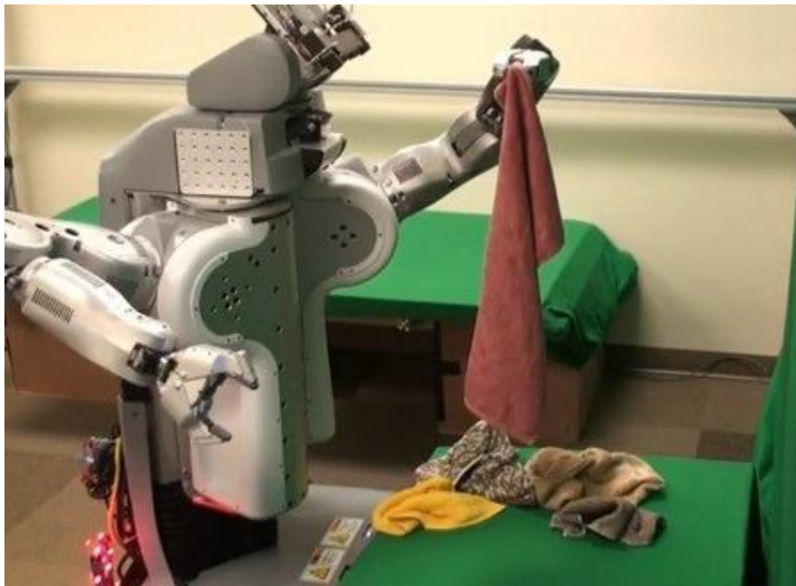
Researchers struggled to train machines to complete tasks like folding towels. Hackaday, 2016, 49
